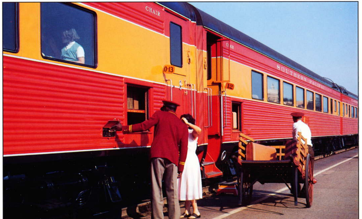
New features of the re-equipped MORNING DAYLIGHT of 1940 included baggage elevators. A car porter at Glendale (RIGHT) operates the controls. Note how the DAYLIGHT color scheme is carried across the exterior of the outer diaphragm at the end of each car. (Bill Olson)
