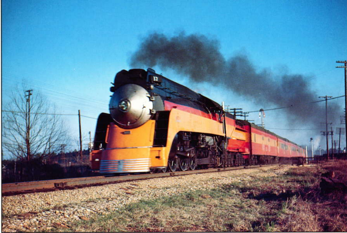
Train 13-14, the SUNBEAM, was entrusted, not to 4-8-4's, which were too large for the turntables on the former Houston and Texas Central, but to three rebuilt 1913-vintage Pacifics. With disc drivers and booster, stream-styling, nose cone, frontal valancing and recessed coupler, the P-14's looked even more bulletlike than the GS-2's. The SUNBEAM made the afternoon run between Houston and Dallas (264 miles) in 4¾ hours, including two stops. When a morning counterpart, the HUSTLER, was established in June 1938 to cater to local traffic, the SUNBEAM became non-stop on a mile-a-minute schedule. With Train No. 14, P-14 No. 652 (LEFT) blazes away from Houston in November 1945. (Emery Gulasch)
