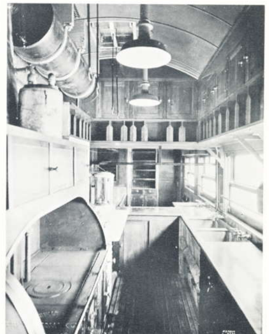
Here is the kitchen area, with the wood or soft coal burning range on the left and the sinks on the right, looking into the pantry section. The tank above is a steam reservoir for the steam cabinet below.
