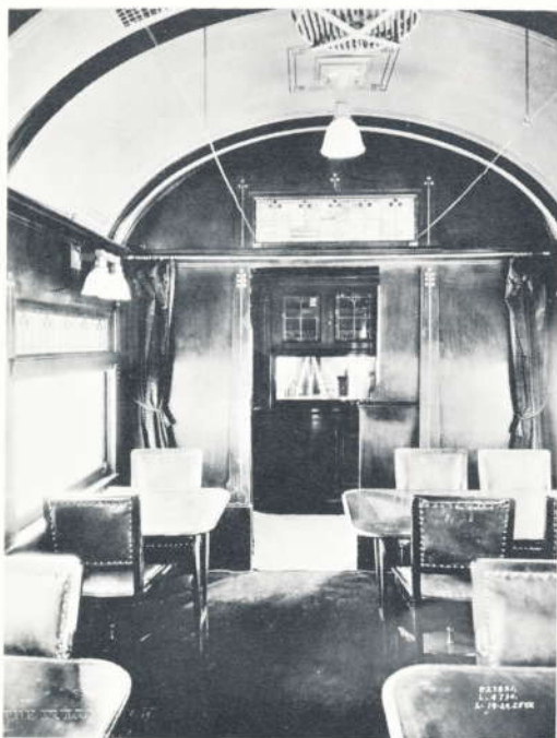
This view is looking forward into the kitchen and pantry from the dining section. These Diners had a seating capacity of 36 passengers. They had six 4-chair tables on the right side and six 2-chair tables on the left.
