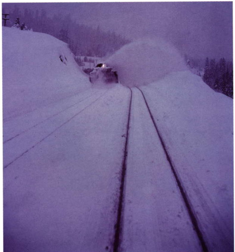
Even during the construction of the Central Pacific, the difficulties of clearing winter snows became very evident. But with the invention of the rotary snow plow, the railroad acquired a powerful weapon against deep snow. In this view, taken on a stormy day, a rotary shows its power, clearing snow from the double track of the Sierra mainline. It was typically possible to throw snow clear across an adjoining track and down the far hillside.
